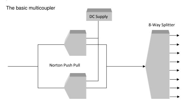
The above diagram shows a multicoupler block diagram. Target specification for such a device follows:-
