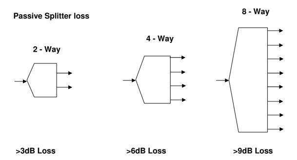
As can be observed, when using a passive splitter, losses to an incoming signal can be guite high. To overcome this generally an amplifier is placed ahead of the splitter. Dependent on the range of frequencies to be split different approaches are taken. The splitting elements themselves tend to have characteristics which limit the band to a range of frequencies that are efficiently split.
